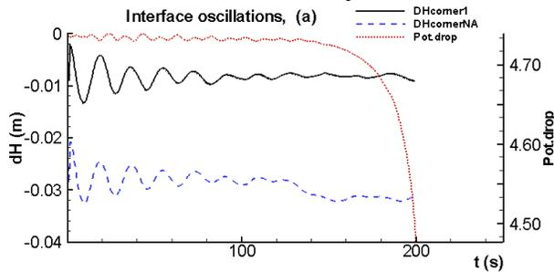
Figure 22. Evolution of the interface position (m)
